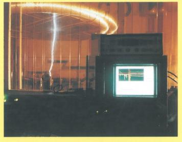
ELECTROATMOSPHERIC CONDENSER: The Apollo has an external housing isolated with regard to its central shaft connected to the earth. Forming a natural condenser in function of the surrounding electric field, with two spark gap, one in controlled atmosphere and another in environmental atmosphere.
